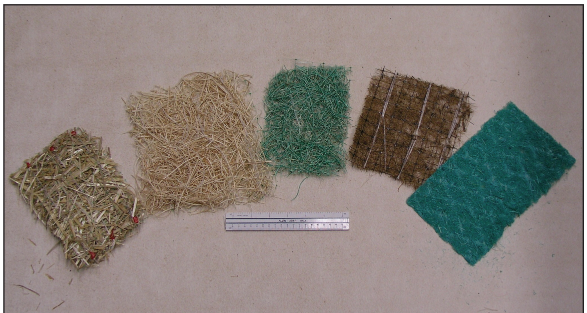
Figure 10—Various erosion control blankets (l to r) – straw, excelsior (natural), excelsior (dyed green), coir, and netless wood/synthetic.
