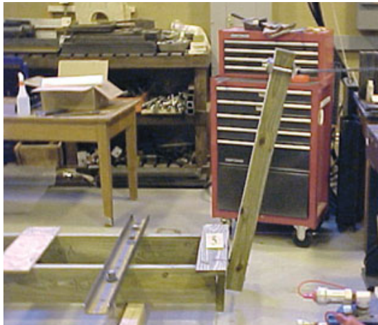
Figure 2. In testing done at Virginia Tech, every traditional wood-to-wood post-mounting detail failed. It wasn't the post-to-rim-joist connection that failed, but the connection of the rim to the deck framing.
